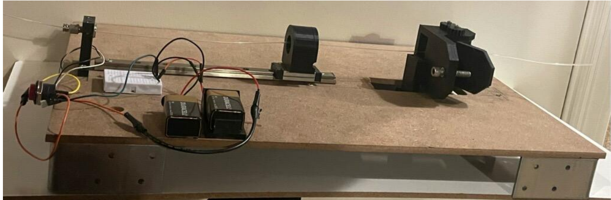
Figure 11: First Iteration of Radial Expansion Tester
